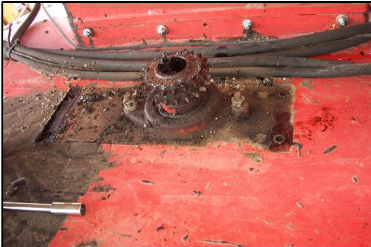
Fig. 6-5 Removal of Motor Mount Assembly
